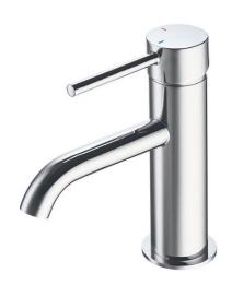
Deck-mounted monobloc basin mixer tap with 91mm lever handle. This basin tap is made from solid brass, and has both hot and cold water connections, with a flow rate of 12.31/min at 1.0 bar pressure.
